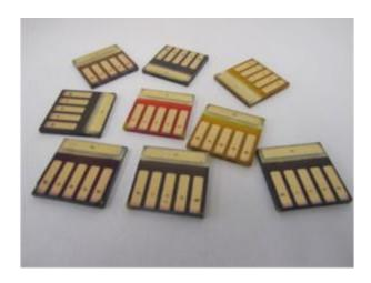
Researchers from the <u>Universitat Jaume I</u> (UJI), in Castelló, Spain, and the <u>University of Oxford</u>, UK, have designed a highly efficient solar cell based on perovskite as light absorber and a combination of titanium oxide and graphene as charge collector. The device, fabricated at temperatures below 150 degrees Celsius, achieved a record efficiency of 15.6% for graphene solar cells.
